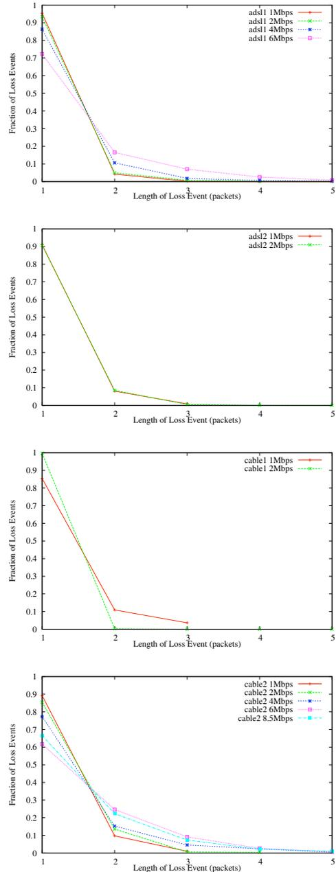
Fig. 3: Distribution of Loss Burst Lengths (packets)
